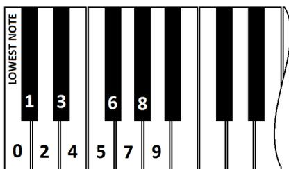
board - refer to master controller chapters at the beginning of this manual. The digits for user settings are at the lowest 10 contact inputs (notes) of any keyboard scanner either internal (MBBS, MIDI128) or external (BBS-1K, BBSP, PDS, DMS-2K) starting with 0 up until 9. Any MIDI keyboard connected to MIDI IN of MRG2 or MIDI128 can
