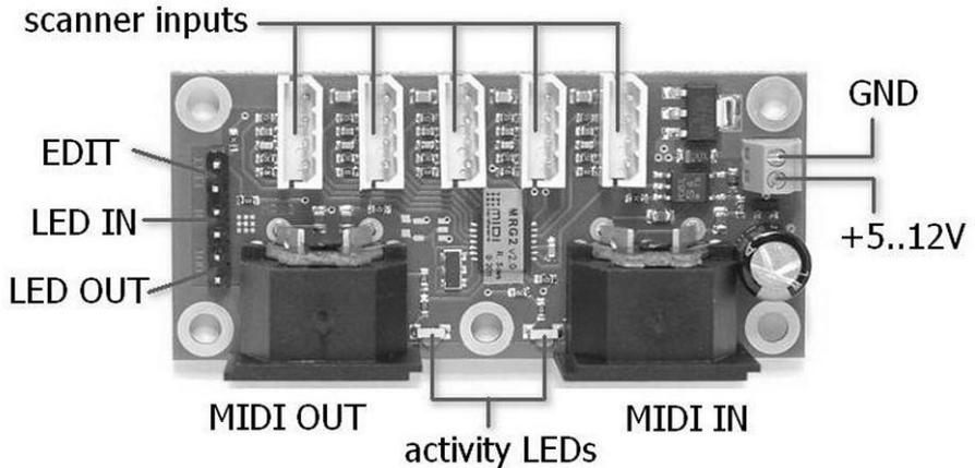
The 6-pin header at the left side of PCB contains connections for external activity LEDs (MIDI OUT and IN) and the EDIT momentary button. The pin out is shown here:
