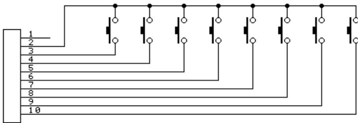
Default configuration of control inputs is described below, with connector layout. All function except the EDIT input (pin 10) are user assignable
