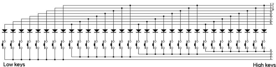
To change note order if it's not correct due to different diode matrix, use the procedure described in chapter 9.2 about DMS-2K (commands #921, #922, #923, #924). To maintain compatibility with currently available master controllers, use PDS in version at least 3.0, otherwise note order setup will not be possible.
