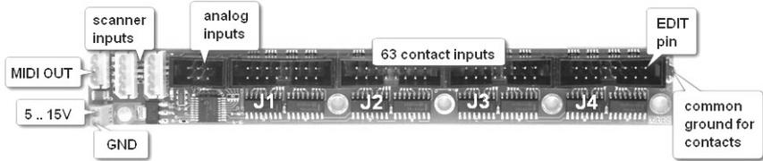
**3-way connector**, depicted in the picture as MIDI OUT matches the cable included with order. It has high quality DIN5 panel mount socket on the other end.
