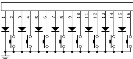
The pins of each LED and buttons connector are interleaved for easier installation. Odd pins are LED outputs, and even pins are button
