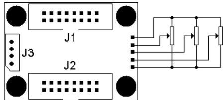
When using pot resistance larger than 20k or wires longer than 30cm, a **shielded cable is required**. The shields of 3 cables (from 3 pots' wipers) should be tied together at the lowest of the 5 pins when oriented as in the diagram here. See chapter 4 for more info on potentiometers usage.
