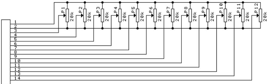
There are 12 inputs for pot wipers, and 2 for top and bottom taps. The pin numbering within one connector is shown here. Notice orientation of the keying slot. If you don't use all potentiometers you may want to connect unused inputs to VCC (pin 1).
