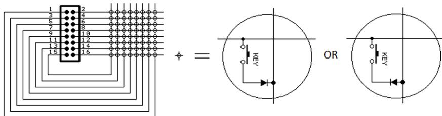
**Automatic diode matrix selection** can be invoked by shorting pins 7, 8, 9, 10 of "special switch inputs" connector at once to GND while the MIDI128 is powered off. Turn the power on for MIDI128 while holding those 4 pins connected to GND. It can be easy done with banana cable connected to GND.
