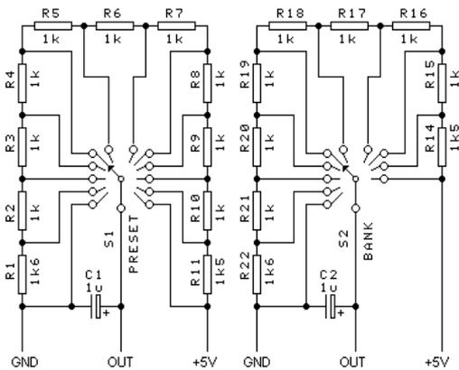
potentiometer, you must add appropriate resistor network around the switch leads, as shown in schematics above.
