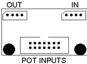
POT12 adds 12 analog inputs (potentiometers or voltages) to MIDI system built around any Master Controller. It has one 14-pin black connectors for potentiometers, and 2 small 4-pin sockets, typical for all scanner boards described here. The one indicated "OUT" goes to Master Controller. The other one can be used to connect another
