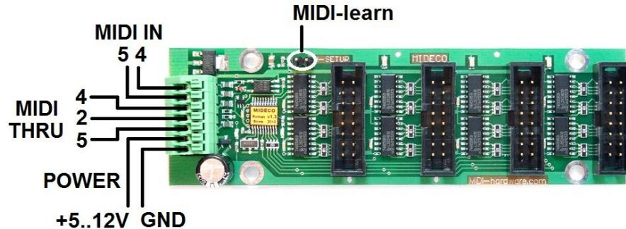
MIDI input is connected with push-in terminals, so no special connectors or tools are needed. MIDI DIN socket should be connected directly, without any components or power in between. If chaining more MIDECO boards, for example to have full 128 note display, you may connect MIDI signal between the 2 boards using plain 2-wire cable, no socket is needed.
