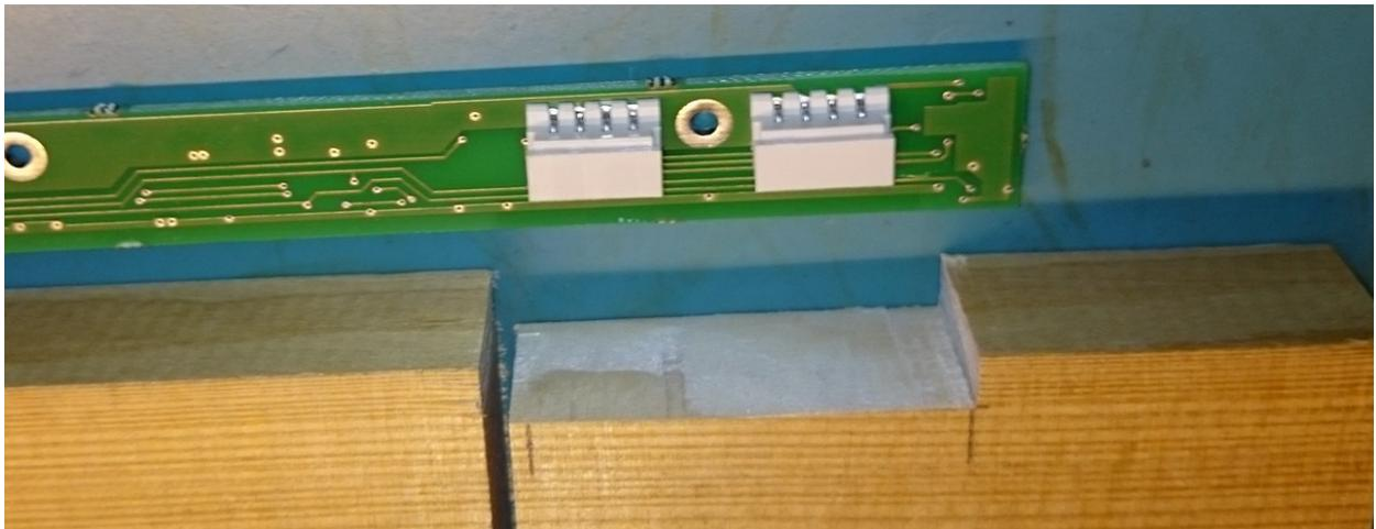
3. Place the board over keys and align all 4 PCBs so the hall sensors (little black thingies) are more or less in the middle of each key. Few milimeters off center is perfectly OK, as long as it's not the edge of a key. Mark PCB locations on the board.
