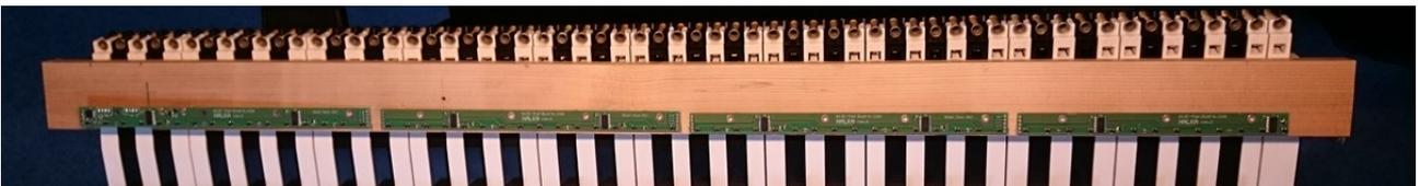
4. Attach all 4 PCBs to the narrow side of wood board, using previously made marks as positioning reference. It may be better to place them in line with bottom edge of the wood, then it's easy to keep all sensor at the same height with respect to keys. Mark hole position and predrill them with small diameter drill bit so it's easier to mount the screws without risking PCB damage.
